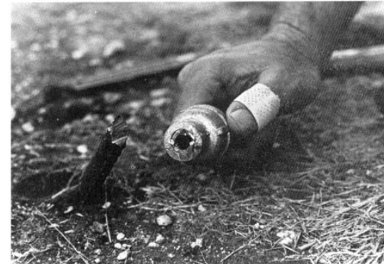
Note the "seat" created in the end of the driver (the 1/4 inch nipple screwed into one of the reducers).
