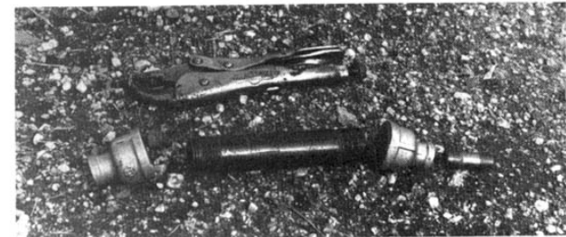
This cheap, easily made tool is necessary for emplacing road spikes. The different parts are shown here in an exploded view. (See text for details.)
