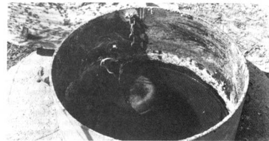
Float-valve regulates water level in stock tank.
